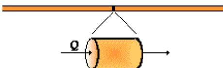
Current is the rate at which charge passes by a point on the circuit. If a small cross section of a wire could be isolated and the quantity of charge ( $Q$ ) passing through this cross section in a certain amount of time ( $t$ ) could be measured, then the current would be the  $Q/t$  ratio.
