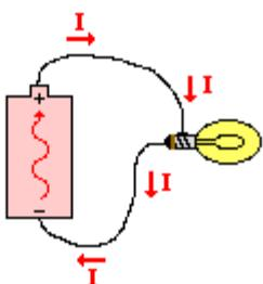
**Electric current in the external circuit is directed from the positive to the negative terminal.**
